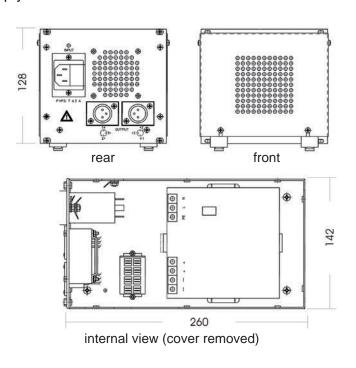
IEC power input connector with fuse-holder
